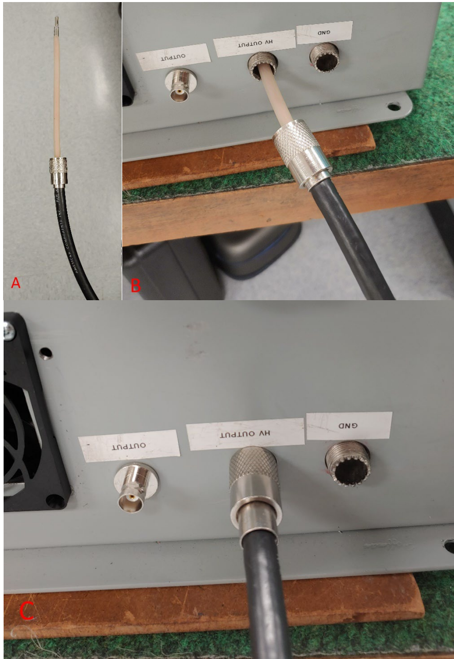
Figure 8 – End of the HV lead on the test chamber (A), inserting it into the HV OUTPUT (B), and inserted (C).
