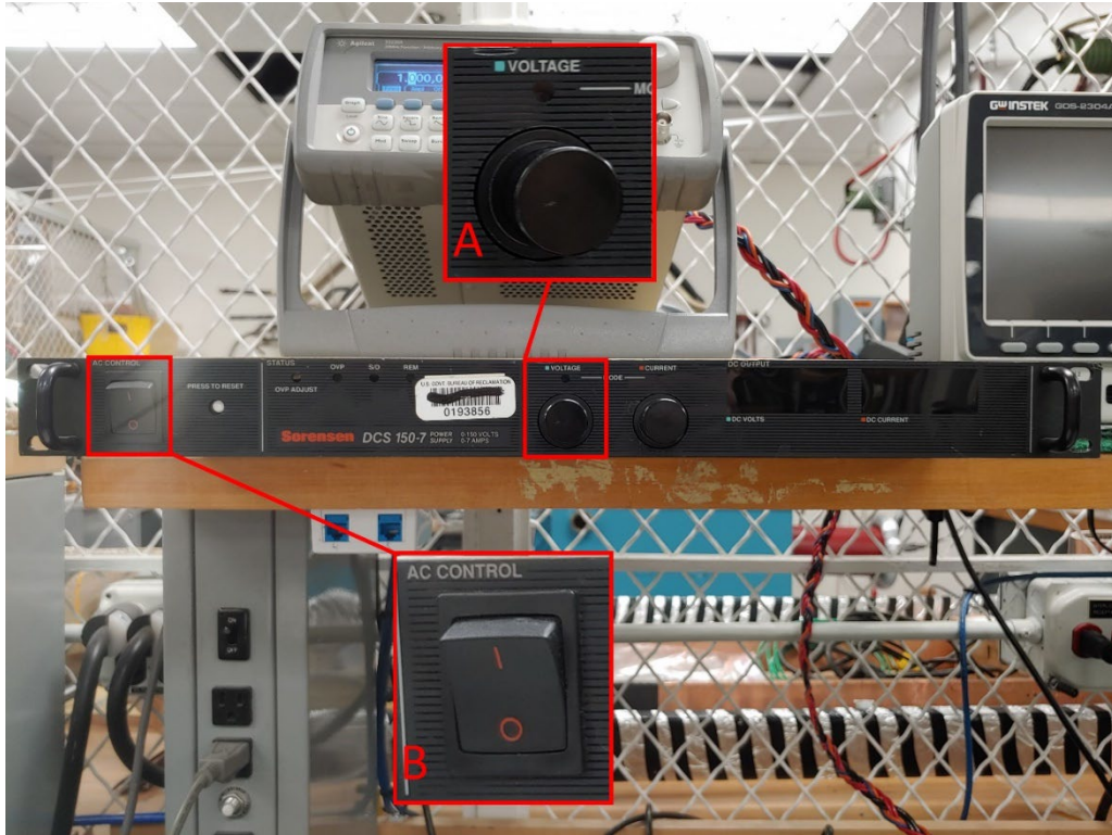
Figure 18 – Voltage knob (A) and power switch in the off position (B) on the DC power supply.
